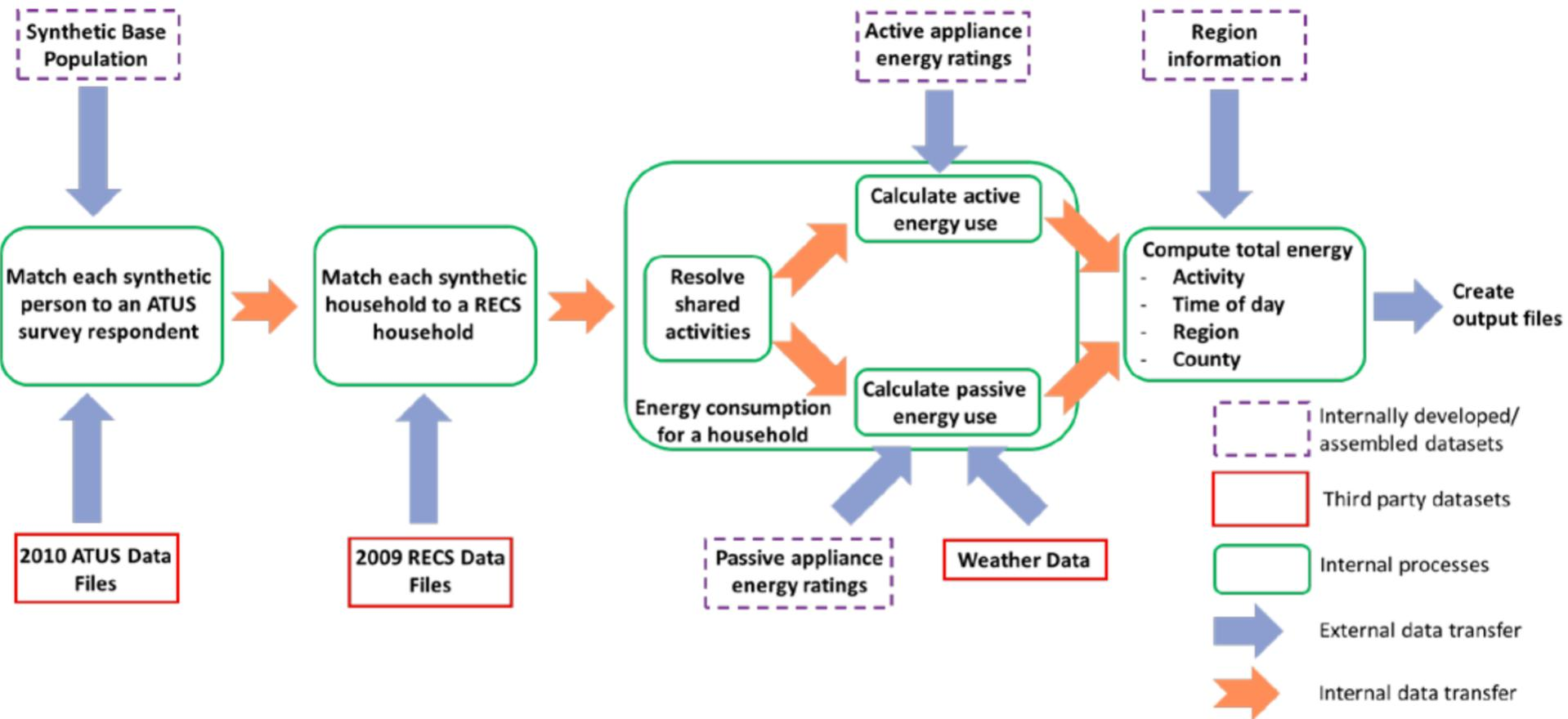
Fig. 2. Modeling framework to generate energy demand model for residential buildings
